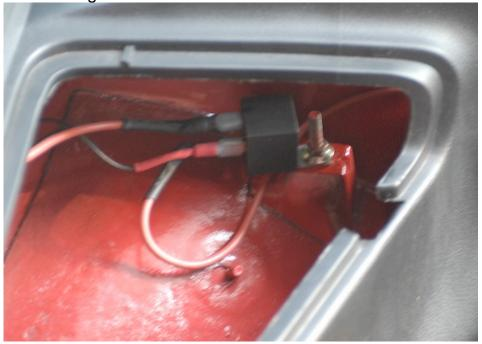
**Image 8** – This shows the white tach wire from the LS1 harness connected to the yellow/blue wire found at B101, the smaller of the two yellow connectors.
