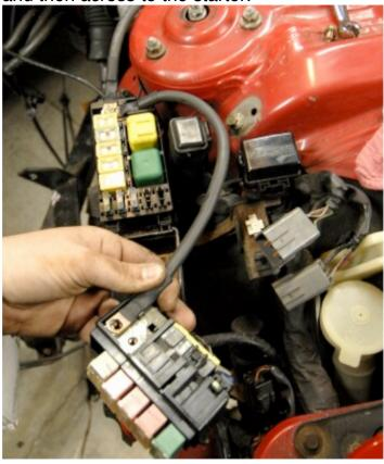
**Image 2** – Black/white switched 12v wire under steering column. 12ga wire to 25 amp fuse then to the pink LS1 harness wire.
